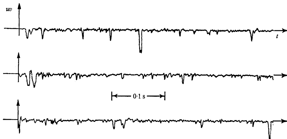
FIGURE 1. The uv component of the Reynolds-stress tensor as function of time at y^+ = 30 . From Willmarth & Lu (1972).
